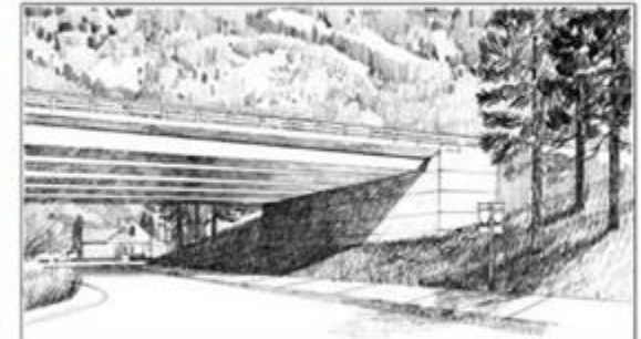
D | Open pedestrian connection, transparent bridge rail, vertical abutment, deep shadow line, and landscape planting strategies.
